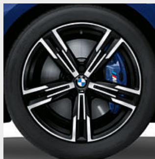
□ 18" M light alloy wheels Double-spoke style 848 M Bicolour Jet Black with mixed tyres, gloss-lathed, wheel size front 7.5J x 18 with 225/45 R18 tyres, wheel size rear 8.5J x 18 with 255/40 R18 tyres. 1,2
