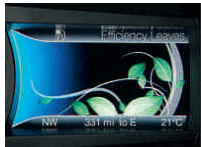
Instant feedback. The more efficiently you drive, the more green leaves appear on the SmartGauge®.
