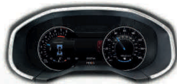
A special display on the cluster panel shows the power distribution between all four wheels. (Standard on all Intelligent All-Wheel Drive models)
